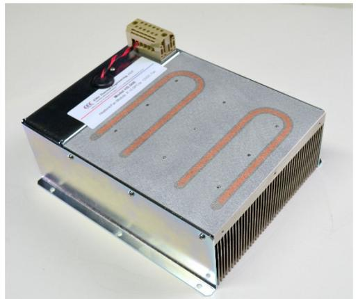
The heatsink used for OCP-150 is our model HS-008. HS-008 has two heat pipes embedded in the base of the heatsink to minimize heat spreading resistance; both heat
